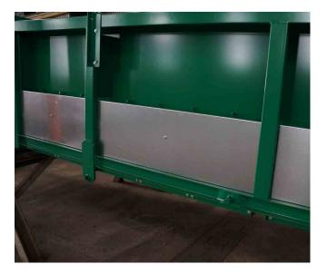
Covering of the profile steel construction made of galvanized sheet metal - can be quickly dismantled
