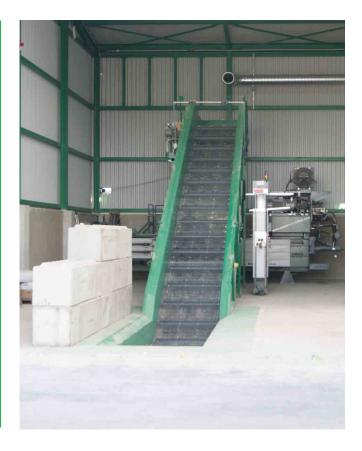
The conveyor technology can be expanded into a material store with an additional increase in the side walls. To fill the belt, a lifting device with a shovel or a grab is required.
