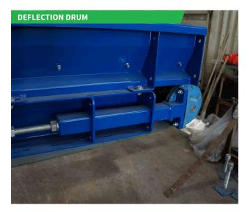
Both the drive as well as the deflector drums are equipped with clamping sleeves and continuous shafts, so that the shaft and the drums can be replaced separately.
